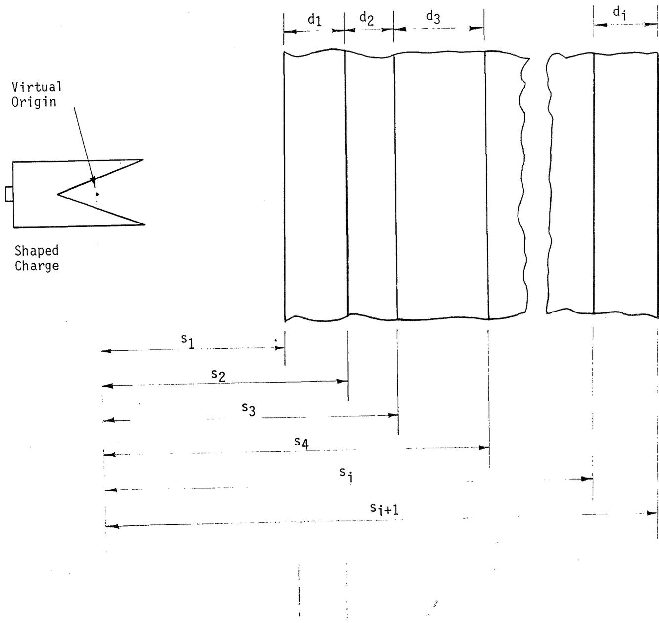
Figure 4. Geometry of a Shaped Charge with Virtual Origin Penetrating a Layered Target.
