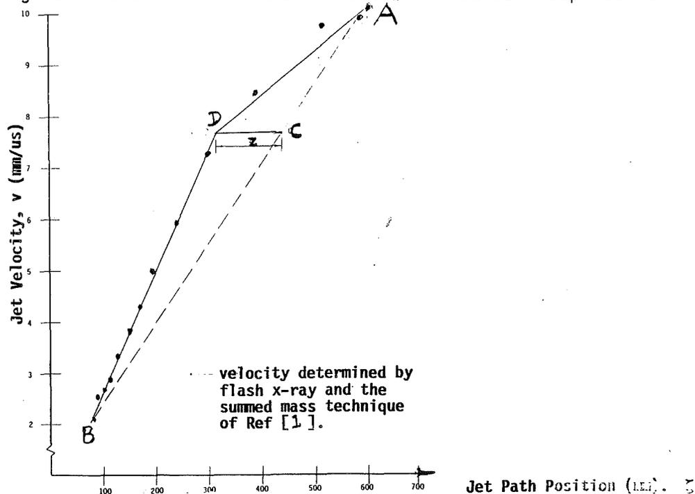
Figure 3. Jet Velocity Distribution of a Biconic-liner Charge, Taken at 100 usec After Detonation.
