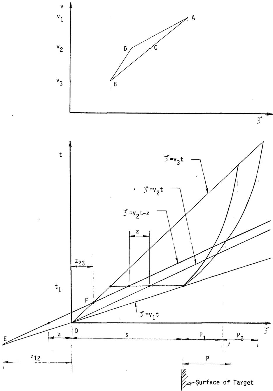
Figure 2. Velocity-Space and Time-Space Diagram of a Jet with Bi-linear Velocity Distribution and their Penetration Curves.
