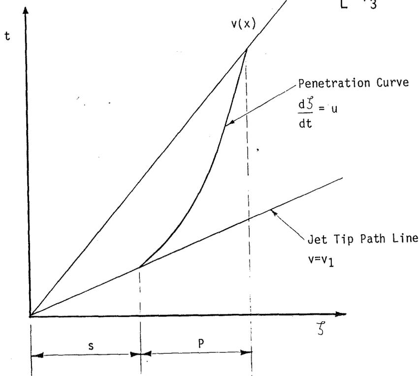
Figure 1. The Jet Particle Path Lines and the Penetration Curve in the Space-time Plane.
