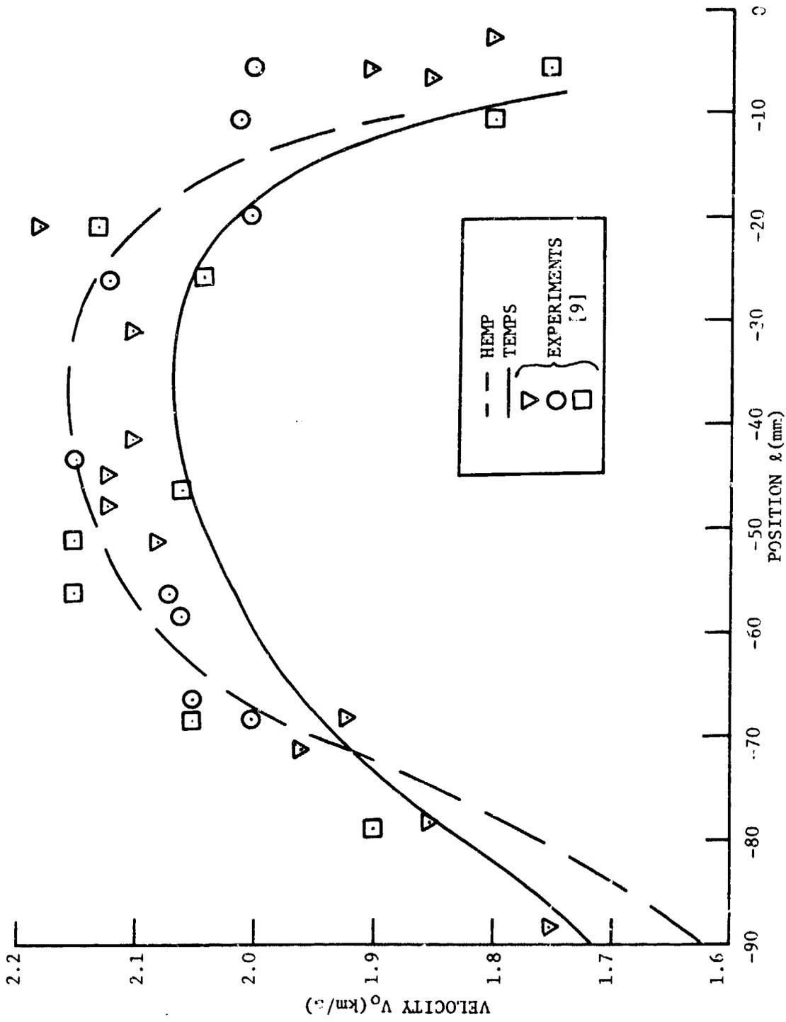
Figure 8. Comparison of TEMPS, HEMP and experimental data for  $V_0$  of an exploding cylinder.
