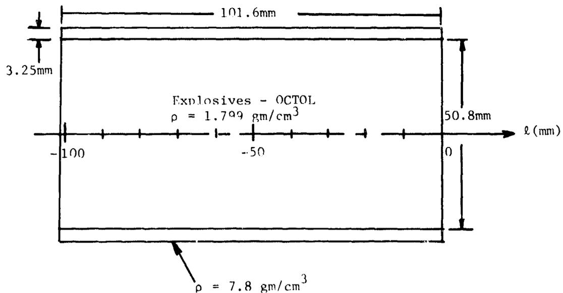
Figure 7. Exploding cylinder charge used for comparisons.
