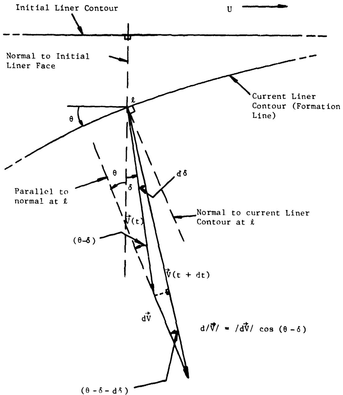
Figure 1. Liner acceleration diagram showing how the additional velocity  $d\vec{v}$  contributes to the increase in magnitude and change in the direction of the current velocity,  $\vec{v}$ .
