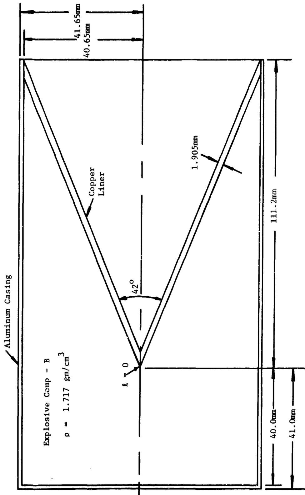
Figure 3. Drawing of 81.3mm diameter  $42^\circ$  conical shaped charge.
